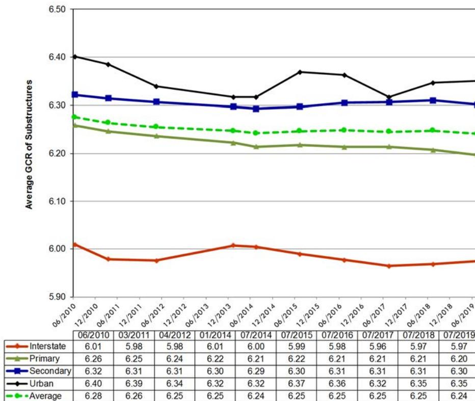
Figure C-4- Substructures: Trends in Average General Condition Ratings by Highway System
