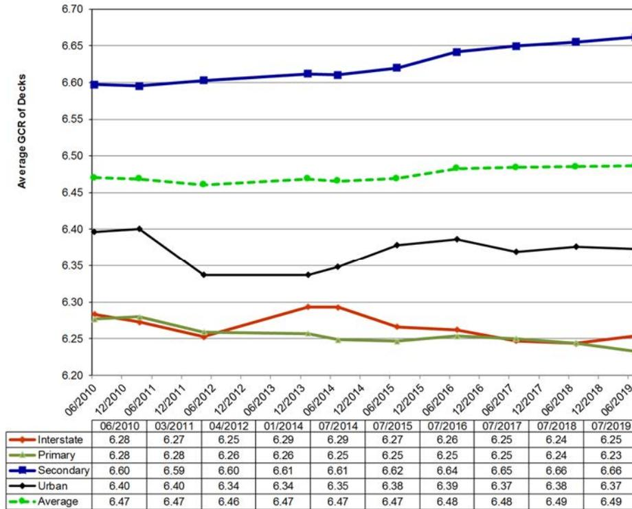
Figure C-2- Bridge Decks: Trends in Average General Condition Ratings by Highway System
