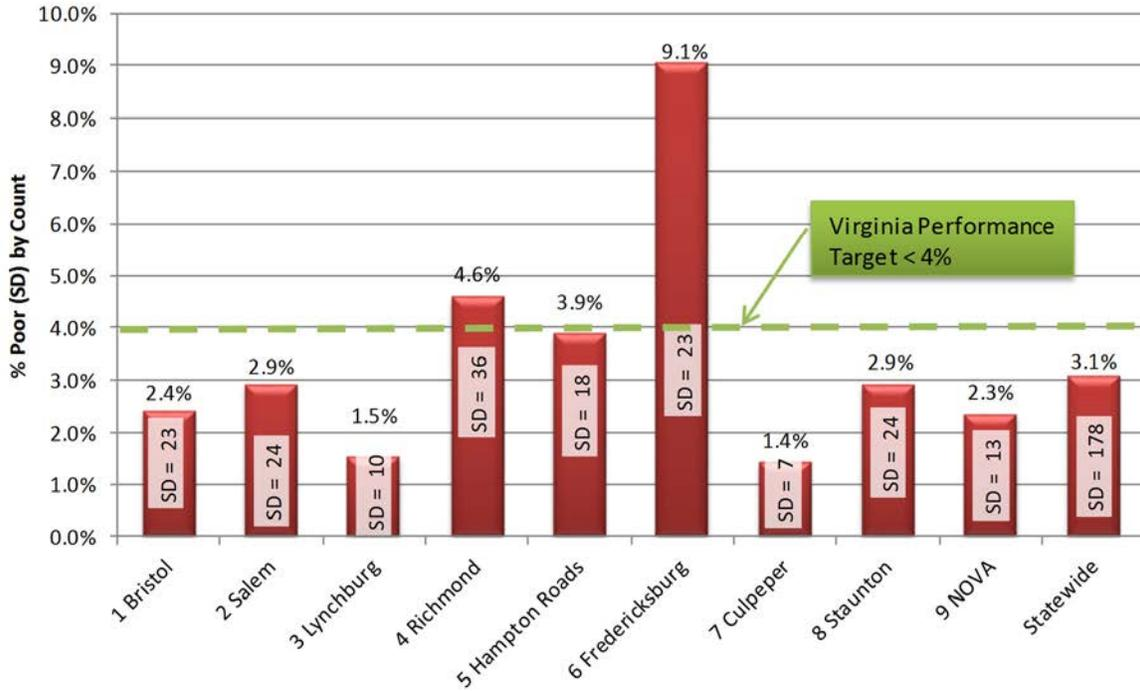
Figure 3-11- Percentage and Count of Poor (SD) Structures on Primary System by District
