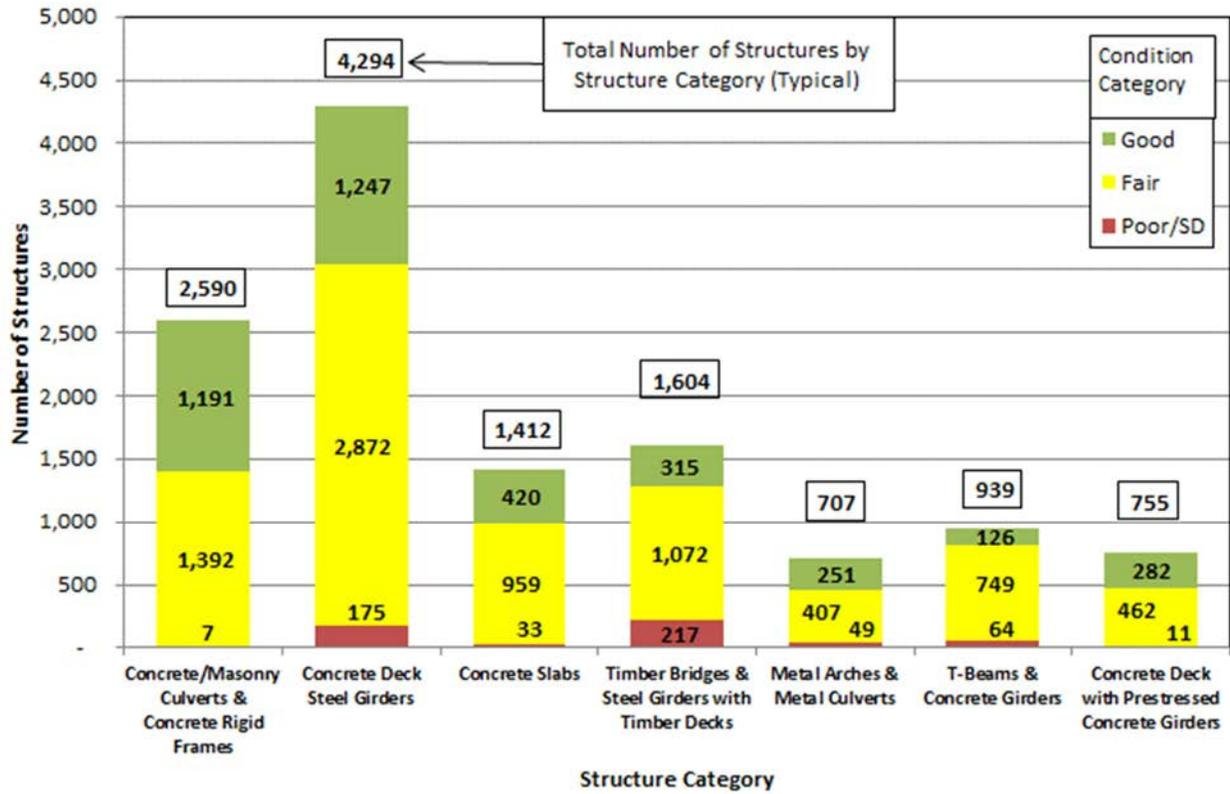
Figure 2-6- Count and Condition Data for Most Common Structure Categories (NBI Structures)
