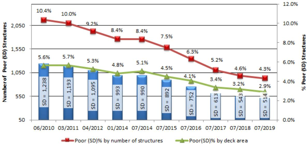
Figure 3-23- Percentage of Poor (SD) Structures - Recent Trends for Secondary System by Year
