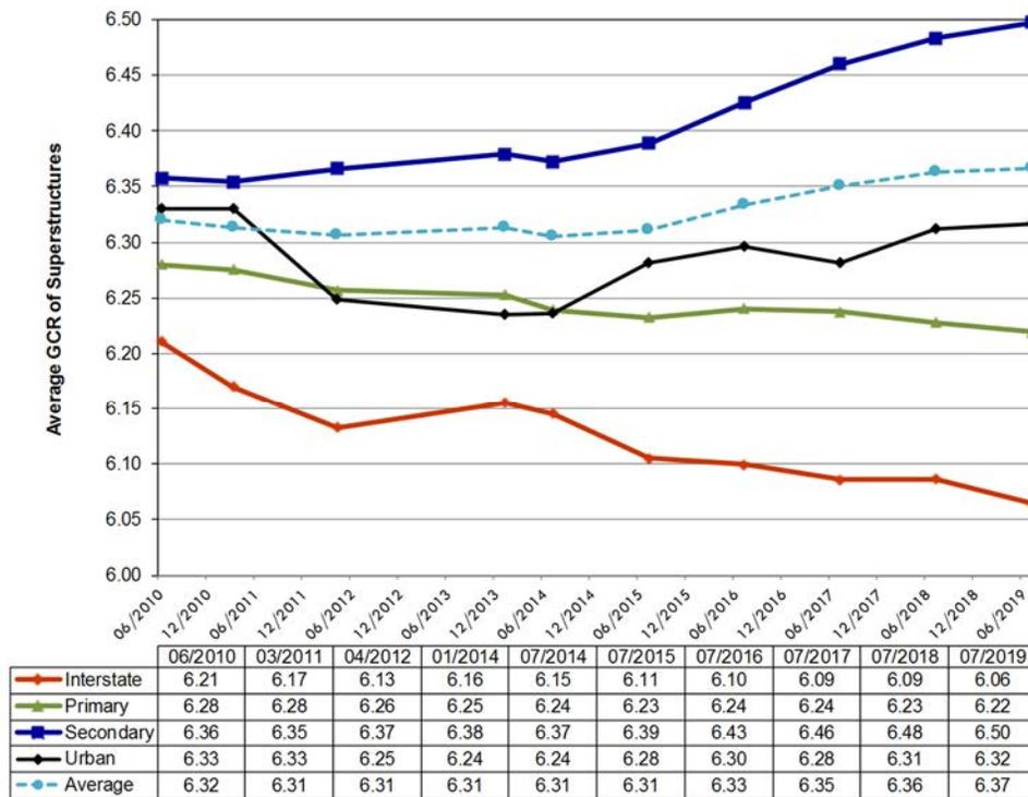
Figure C-3- Superstructures: Trends in Average General Condition Ratings by Highway System
