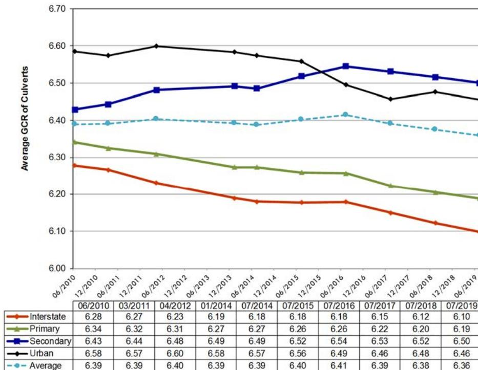
Figure C-5- Culverts: Trends in Average General Condition Ratings by Highway System
