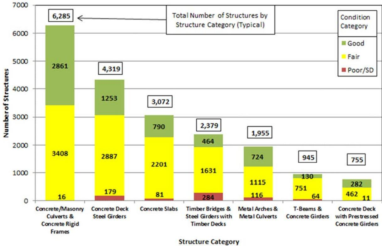
Figure 2-4- Count and Condition Data for Most Common Structure Categories (All Structures)
