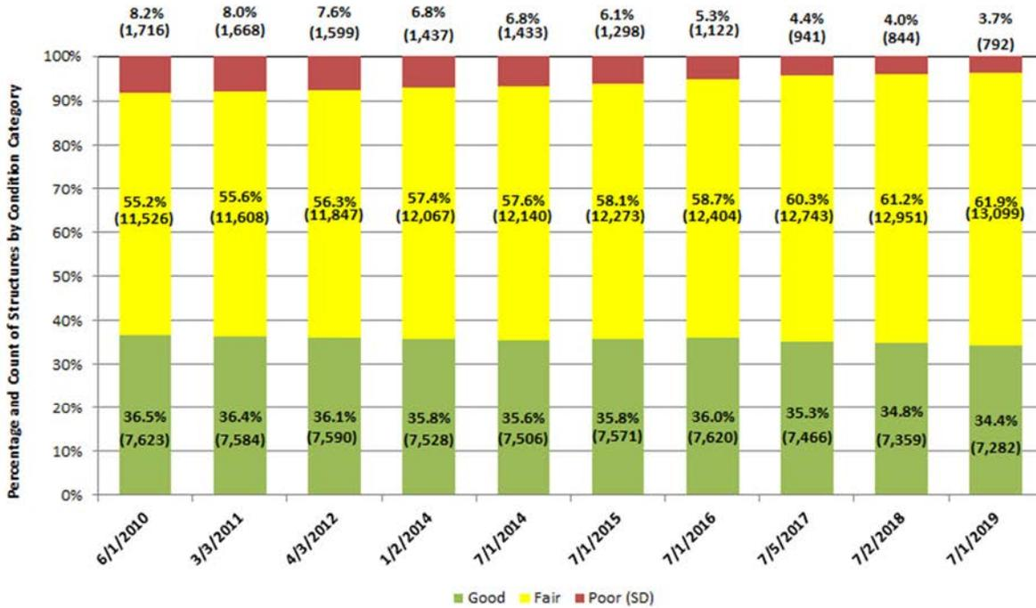
**Figure 3-1: Percentage and Count of Structures in Good, Fair, and Poor (SD) Condition by Year**
