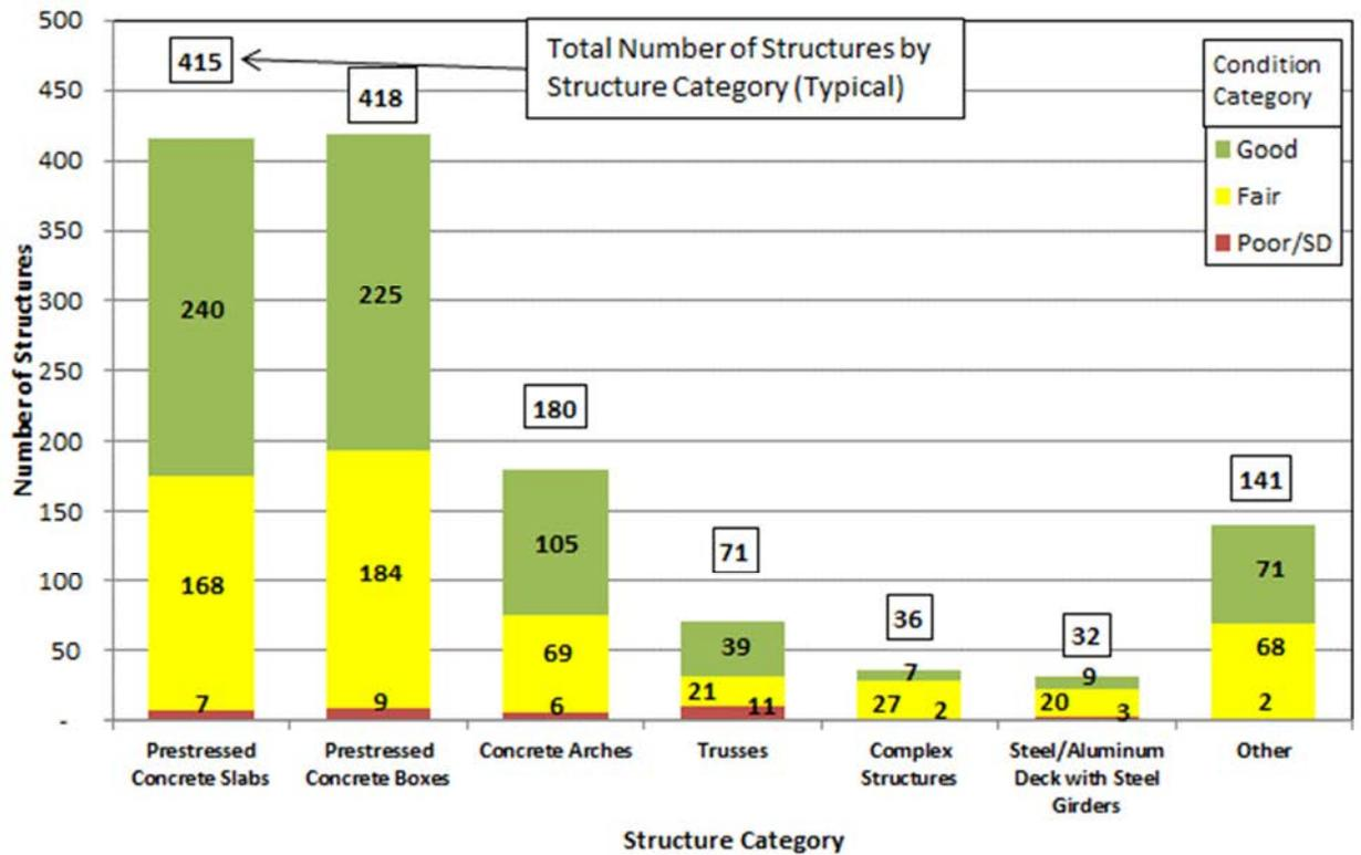
Figure 2-7- Count and Condition Data for Less Common Structures Categories (NBI Structures)
