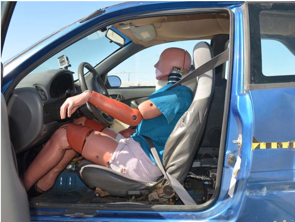
FIGURE 48. Post-Test View of Driver's Side Occupant Compartment
