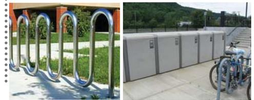
Examples of a 'rolling' bike rack (left) and bike lockers at a transit station (right).
