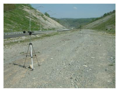
Figure 35. Sound level meter setup on the Smart Road.
