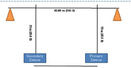
20 m (65.6 ft) Figure 34. Sound Level Meter setup on Smart Road.
