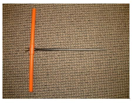
Figure 12. Increment borer for growth ring counting.
