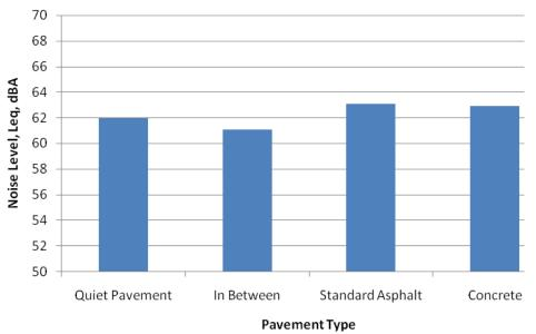
Figure 39. Effect of pavement type on road noise.
