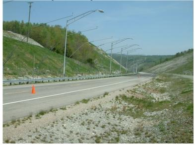
Figure 33. Area 200 feet long marked with cones for measurements on Smart Road.
