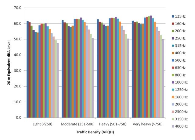
Figure 17. 1/3 octave band measurements from 125-4000 Hz for four levels of traffic density.
