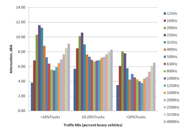
Figure 29. 1/3 octave band road noise attenuation from 125-4000 Hz for four levels of traffic mix (attenuation at 65.6 ft into the stand of trees).
