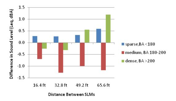
Figure 20. Difference in sound level by tree density, adjusted for expected attenuation due to the distance between the sound level meters (with density categorized as basal area).
