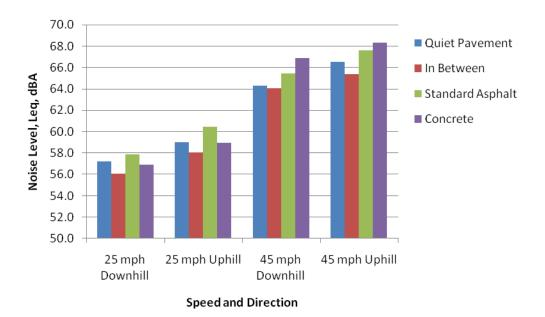
Figure 44. Effect of traffic speed and direction on road noise.
