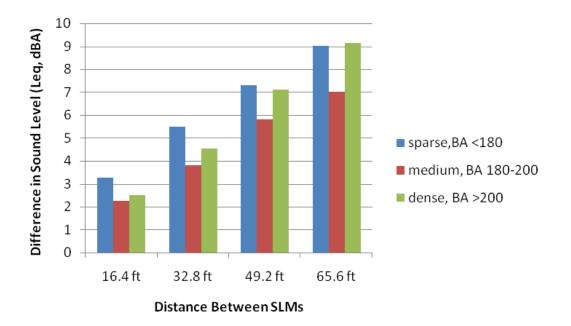
Figure 18. Difference in sound level by tree density (with density categorized as average basal area).
