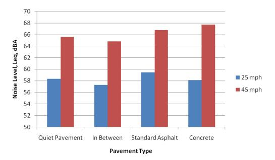
Figure 40. Effect of traffic speed on road noise.
