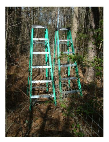
Figure 7. Ladder setup for climbing VDOT fences.
