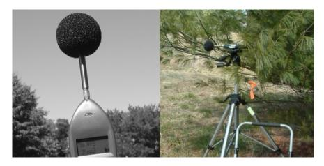
Figure 6. Use of windscreen on an SLM.
