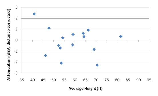
Figure 23. Plot of average tree height by attenuation (distance corrected).
