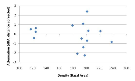
Figure 21. Plot of density (basal area) by attenuation (distance corrected).
