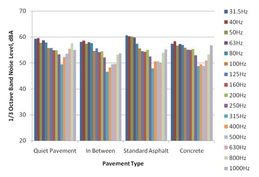
Figure 46. Effect of pavement type on 1/3 octave band frequencies between 31.5 Hz and 1000 Hz.
