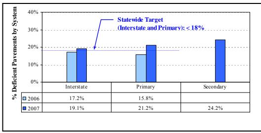
Figure 1. Statewide Percent Deficient Pavements by System
